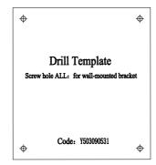
Step 2: Attach the drilling guide template to the wall and drill holes according to the positions indicated on the template. The recommended drilling specifications are a hole diameter of  $\phi$  10mm and a depth greater than 60mm.
