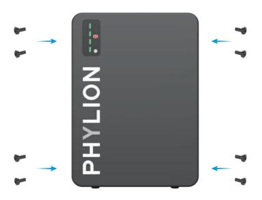
Step 4: Mount the battery pack onto the bracket using 8 M5 screws from the accessory kit. Tighten the screws to a torque of 2.5 N.m.
