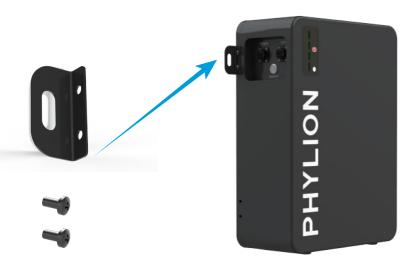
Step 2: Secure the bracket to the battery pack using 2 M5 screws from the accessory kit. Tighten the screws to a torque of 2.5 N.m.
