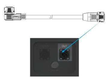
Step 2: Connect additional power and communication cable to the "OUT" port on this battery and the other end to the "PCS/IN" port on another battery(Only For Multiple Batteries Paraller Use).
