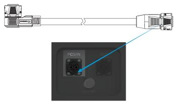
Step 1: Connect the power and communication cable to the "PCS/IN" port on the battery and the other end to PCS.
