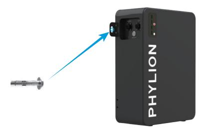
Step 3: Determine the mounting points for the expansion bolts based on the placement location of the battery pack. The recommended drilling specifications are a hole diameter of  $\phi 10 mm$  and a depth greater than 60mm. Once drilling is complete, use expansion bolts to securely attach the battery pack to the wall.
